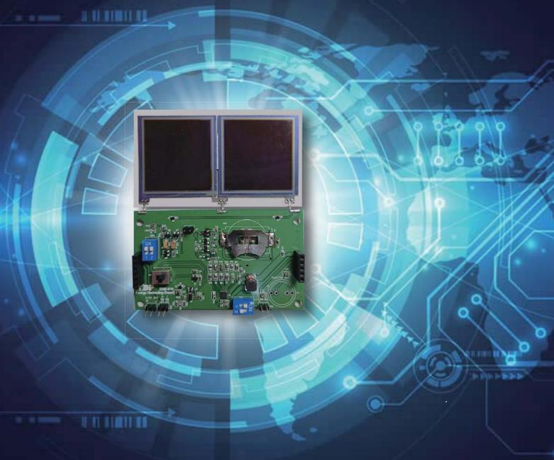
This is a Energy Harvesting Board specially designed for DSC. It's MPPT (Maximum power point tracking) function can efficiently manage the power generated by DSC. The output power is DC 3V/5V switchable and automatically switched over to CR2032 battery when the stored power is low.
